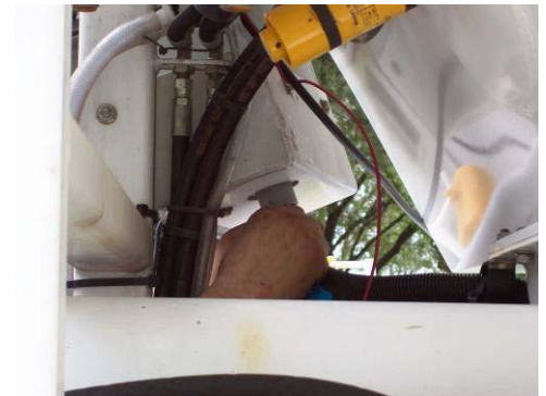
Make an opening in the plastic tube where there are all wires that enter the control panel.
