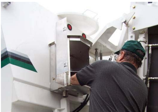
Position the compressed air faucet and fix it with the bolt.
