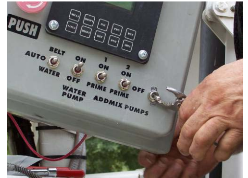
Fix the switch by screwing the nut.
