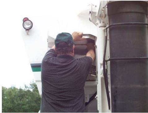
Position the 4 discs and tighten the nuts.
