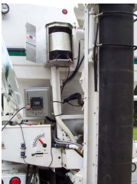
Load the VM AR glass fiber roving
