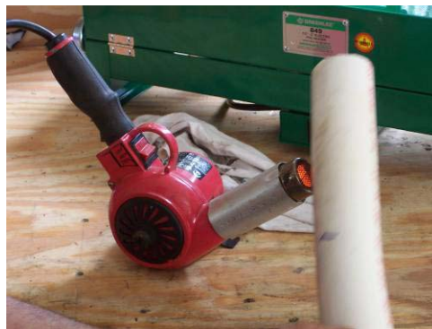
Heat the PVC tube and bend it ...
