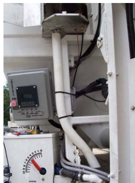
Heat the PVC tube and bend it ...
