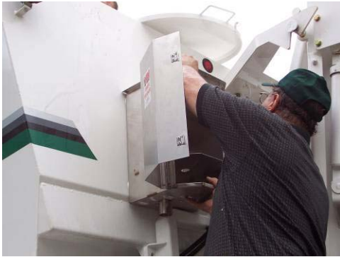
Position the box and ask someone else to put the bolts in the 4 holes.
