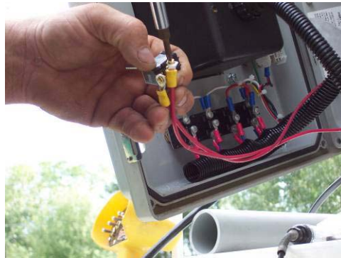
The second wire connected to the switch comes from the material control switch (the switch which controls the belt and the feeding of sand, aggregate, cement and water).
