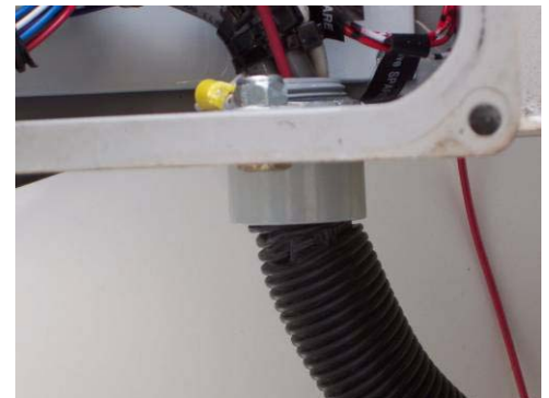
Make an opening in the plastic tube where there are all wires that enter the control panel.
